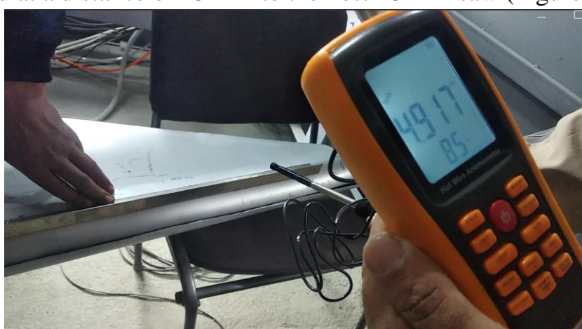
6-Fig. The air gap system is 5 mm and the distance to the saw tooth is 65 mm The air-push system showed 49 meters/second at a distance of 65 mm to the notch 5 mm saw.
